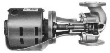
Proven Pump Construction • One piece dynamically balanced impeller • Stainless steel shaft • Rugged bronze sleeve bearing • Two-piece carbon/ceramic seal assembly • Durable one-piece spring coupling.
